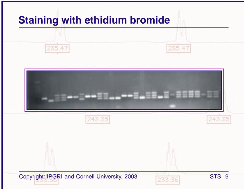
As mentioned previously, one way of visualising microsatellites is by using agarose gel electrophoresis. This method is appropriate when the alleles are long enough, that is, more than 200-300 base pairs, and the differences among alleles also significant (i.e. more than 10-20 bp).
