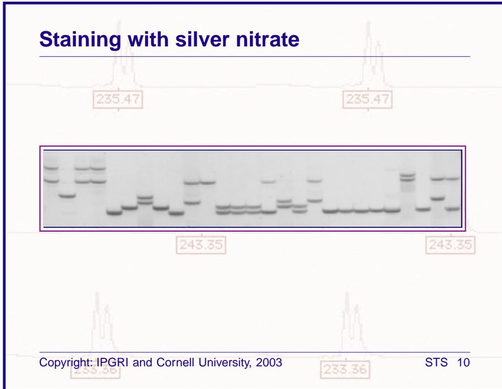
Microsatellites can also be analysed after running PCR products through an acrylamide gel stained with silver nitrate. In this picture, individual samples belong to a diploid species and therefore have a maximum of two alleles.
