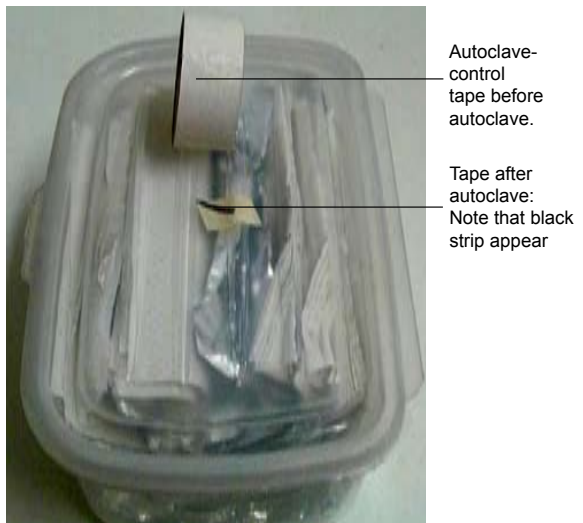
Figure 32. Aluminium and paper foil packed for autoclave
