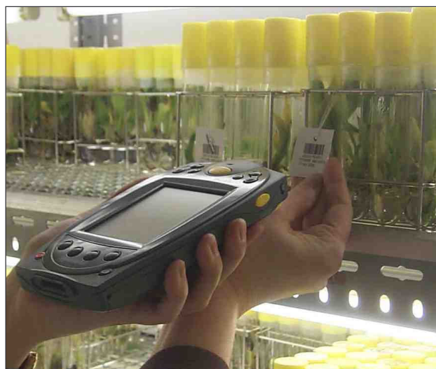
Figure 2. Managing the inventory of the active in vitro collection at the INIBAP gene bank using a barcode based system.
