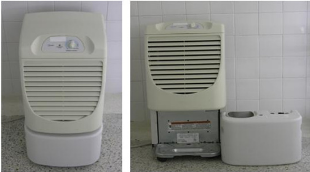
Figure 10. Dehumidifiers used to control relative humidity of the air in the growth and conservation rooms.
