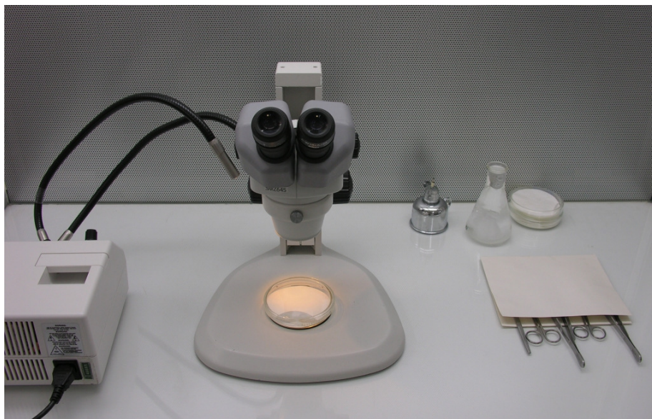
Figure 19. Stereomicroscope and tools required for the isolation of the meristem.
