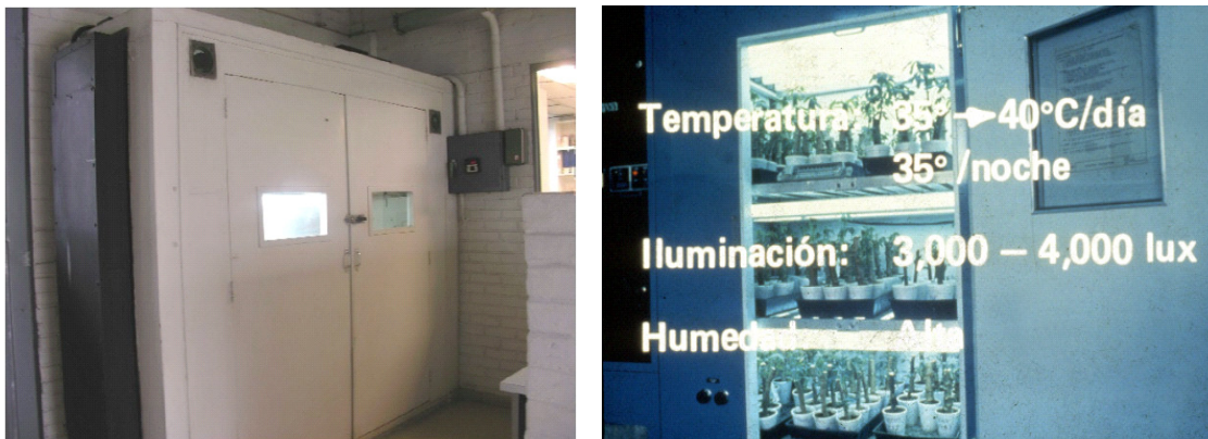
Figure 16. Chamber and required conditions for the thermotherapy process of the stakes.
